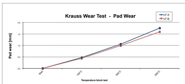
Figure 7: Pad wear comparison after SAE J2707 wear testing
