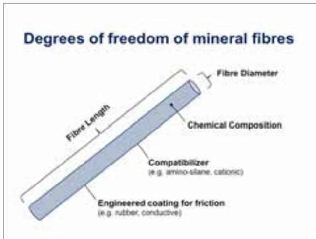
Figure 3: Mineral fibre characteristics
