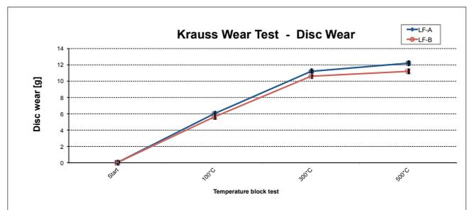
Figure 9: Disc wear comparison after SAE J2707 wear testing
