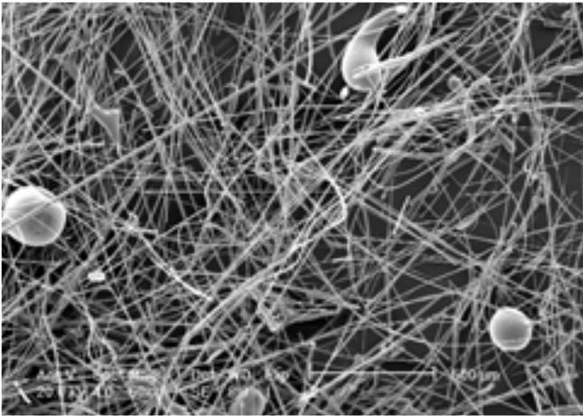
Figure 2: SEM image of mineral fibres before shot removal
