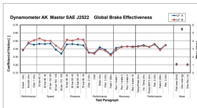
Figure 5: AK-Master efficiency summary comparison
