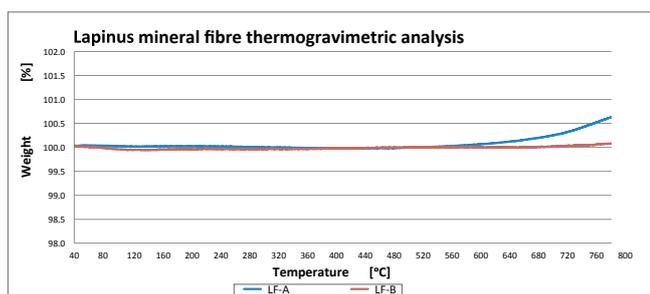
Figure 4: mineral fibre TGA curves, existing versus new fibre grade
