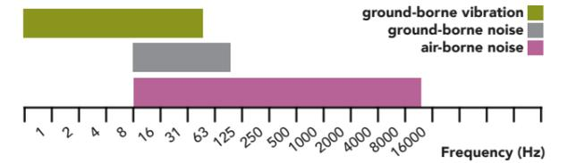
Rockdelta enables an optimal reduction of vibration in a range from 16 up to 120 Hz, depending on the project specific conditions and frequency.
