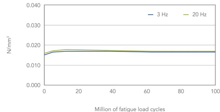
The graph on the left virtually shows zero long-term variation of the low frequency dynamic bedding modulus at 3 Hz and 20 Hz on a Rockdelta® RX mat after 100 million cycles.
