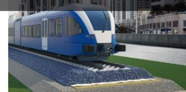
A dual-density sub-ballast mat made up of a low-damping, soft and resilient bottom layer and a high-density, force-distributing top layer.
